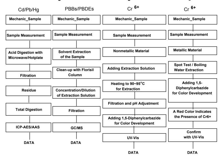
The samples were dissolved totally by pre-conditioning method according to above flow chart for Cd,Pb,Hg.
